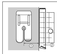
When sewing a margin wider than 7 mm ①, you may find it helpful to attach a piece of tape to the needle plate ② to help guide the fabric.
