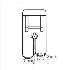
It is convenient to use the markings on the presser foot as a guide when sewing narrow seam allowances, decorative stitches, etc.
